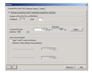
After the general network settings have been finished, double click the slave (encoder) whose parameters shall be set and select the tab "Clocking".
