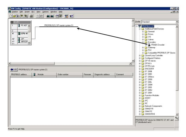
After inserting the Profibus master system into the hardware configuration ("Insert" – "Master System") the FRABA encoder can be chosen from the hardware catalogue and added to the profibus network: Select the device "FRABA Encoder" and drag it with the mouse to the network (or choose the network and double click the "FRABA encoder").
