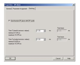
After all Slaves have been configured and all parameters have been set, the general parameters for the whole network (e.g. "Constant DP cycle") should be checked once more (and adapted if necessary).
