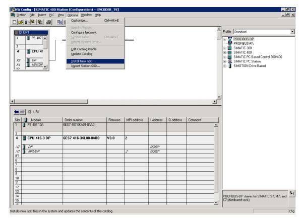
After successful installation of the GSD file the encoder can be found in the hardware catalogue in
