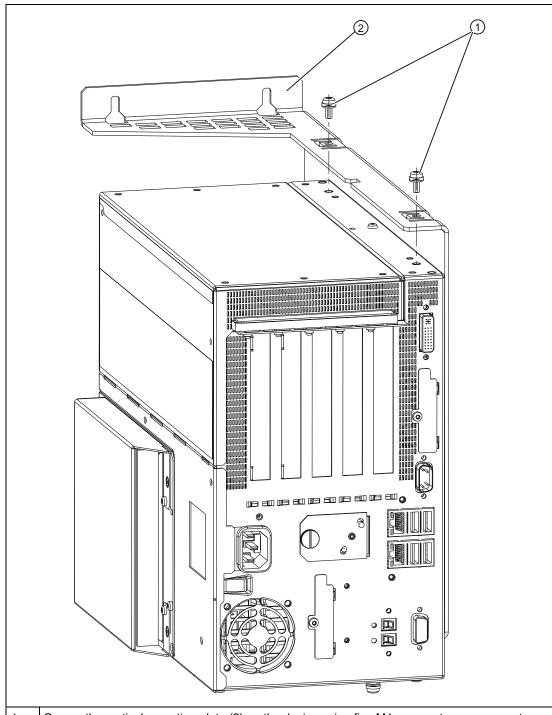
1. Secure the vertical mounting plate (2) on the device using five M4 screws: two screws on top (1) and three (not shown in figure) on the bottom of the device.
