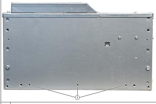
Mount the brackets onto the device using the included M3 x 5 mm screws with a max. insertion depth of 5 mm (included in package).
