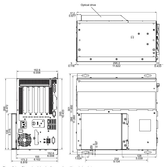
Figure 8-1 Dimensional drawing for mounting with angle bracket
