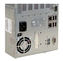
Fasten the cable with the supplied power plug latch, if necessary (1).
