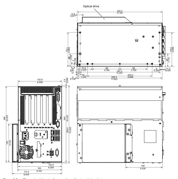
Figure 8-2 Dimensional drawing for mounting without angle bracket
