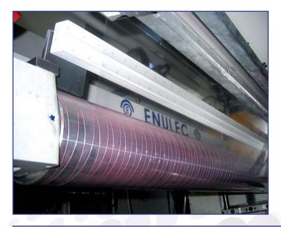
Due to this special design no sparks can occur even if the discharge bar is contaminated with non conductive ink. The discharge bar is not only safer because the build-up of conductive bridges between the needles can not longer occur; it also very significantly lengthens maintenance intervals for cleaning.
