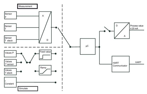
Figure 7-18 Block diagram of simulation
