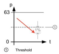
Figure 8-8 Monitoring of a minimum pressure
