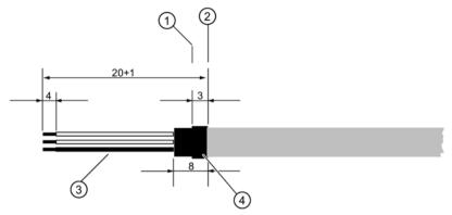
Figure 5-3 Preparing the connecting cable
