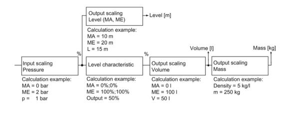
Figure 7-3 Functions of the "Level" block
