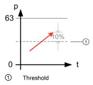
Figure 8-9 Monitoring of a maximum pressure
