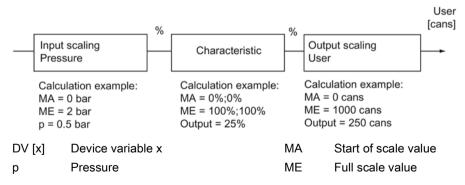
Figure 7-7 Functions of the "User" block
