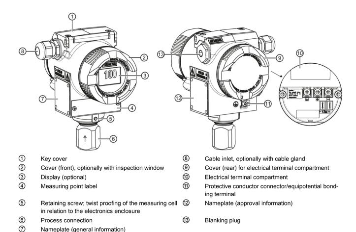
Figure 3-2 View of the pressure transmitter: Left: Front right: Rear view
