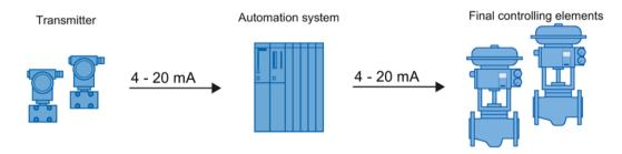
Figure 8-2 Safety-instrumented system in multi-channel operation
