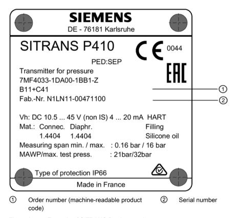
Figure 3-4 Example of SITRANS P410 nameplate
