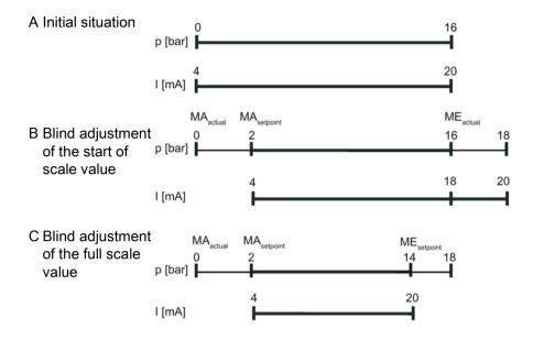
$\begin{array}{lll} I & \text{Output current} & p & \text{Pressure} \\ \text{MA}_{\text{actual}} \text{ Old start of scale value} & \text{MA}_{\text{target}} & \text{New start of scale value} \\ \text{ME}_{\text{actual}} \text{ Old full scale value} & \text{ME}_{\text{target}} & \text{New full scale value} \\ \end{array}$
