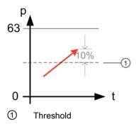
Figure 8-6 Monitoring of a maximum pressure
