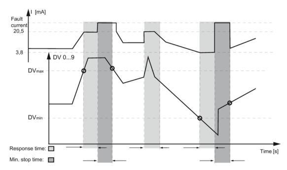
Figure 7-19 Trip levels for the limit monitor
