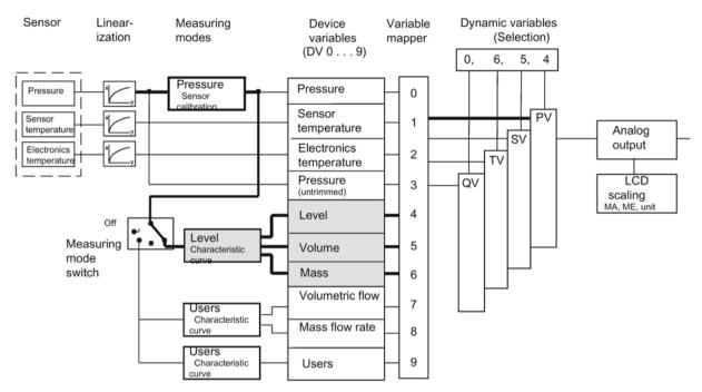
Figure 7-2 Measuring mode "Level"
