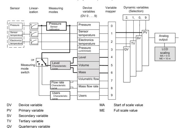
Figure 7-11 Free LCD scaling
