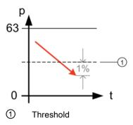
Figure 8-5 Monitoring of a minimum pressure
