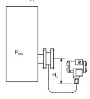
Pressure transmitter for absolute pressure always below the measuring point:  $H_1 \ge 200$  mm (7.9 inch)
