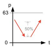
Figure 8-7 Example of two-point measurement 50%
