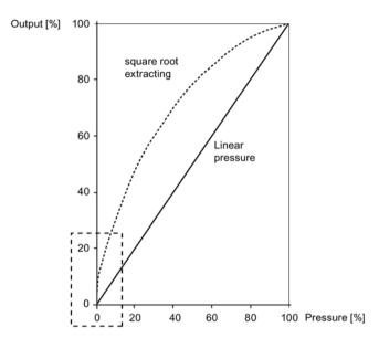
The dotted rectangle has been magnified in the form of the following characteristic curves in order to show the behavior of characteristic curves.
