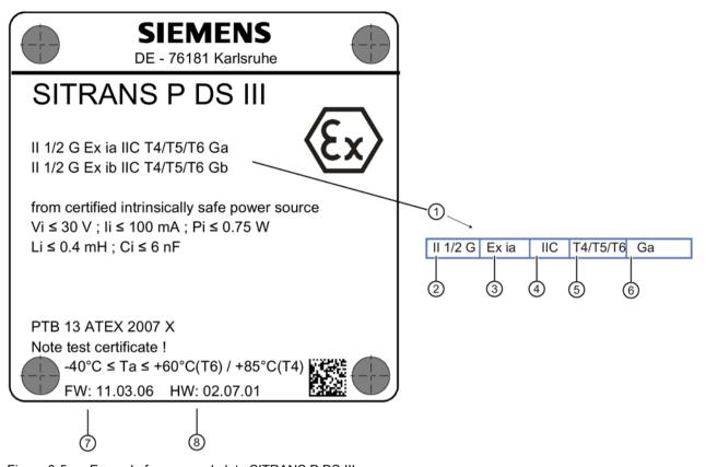
Figure 3-5 Example for approval plate SITRANS P DS III
