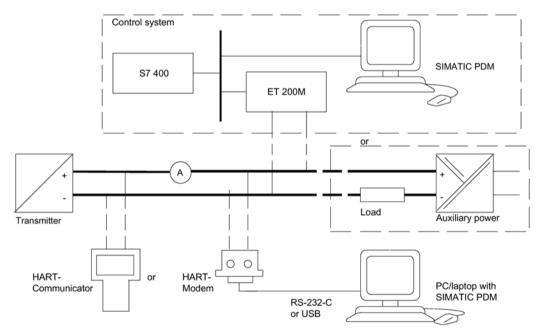
Figure 3-1 Possible system configurations
