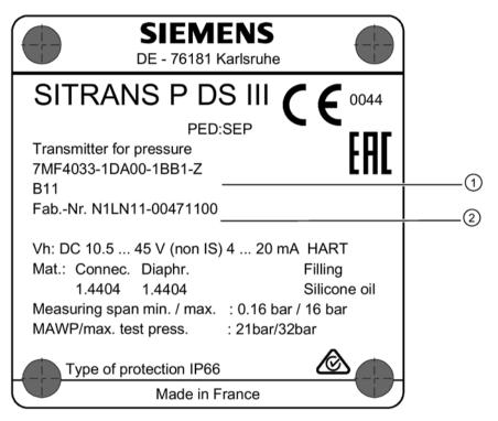
Figure 3-3 Example of SITRANS P DS III nameplate
