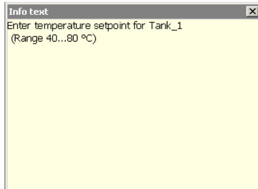
Figure 8-4 Info text for an IO field, example
