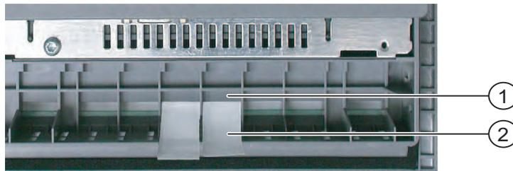
6. Slide the labeling strips into the guide up to the stop.
