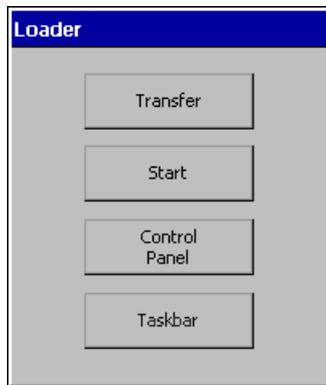
The HMI device automatically switches to "Transfer" mode during initial startup under the following conditions:
