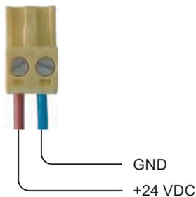
Do not confuse the lines. Refer to the label for the contact pins on the rear of the HMI device.
