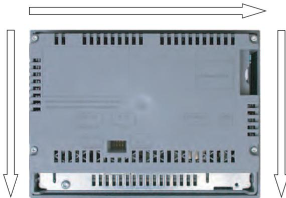
The following table shows the positions of the mounting clamps on the TP 277. Please note the counting direction. The position indicated corresponds to the first recess occupied for each mounting clamp in the counting direction. The inserted mounting clamp covers several recesses.
