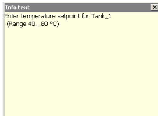
Figure 8-6 Info text for an IO field, example
