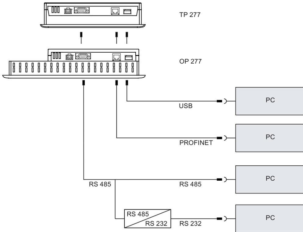
Use a cross-cable for the PROFINET connection when using a point-to-point connection.
