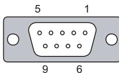
Figure 12-2 Pin assignment of the RS 422/RS 485 interface
