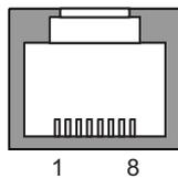
Figure 12-4 Pin assignment of the RJ45 connector
