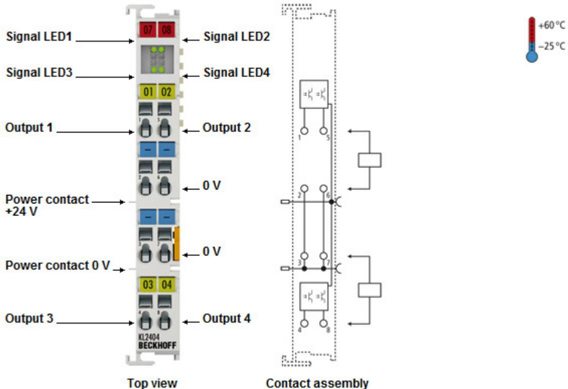
**KL2404, KL2424 | 4-channel digital output terminals 24 V DC**
