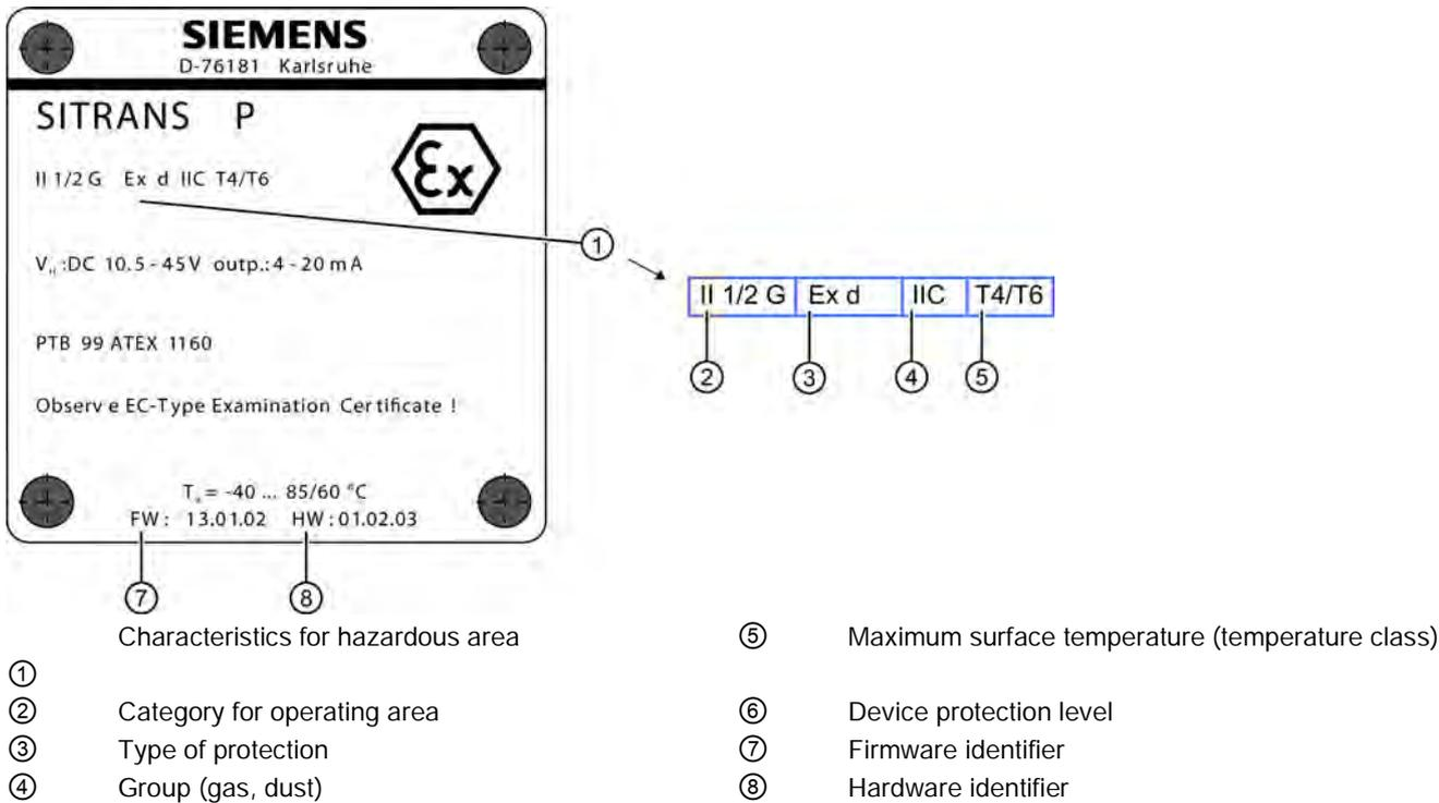
Figure 1-2 Example of a nameplate
