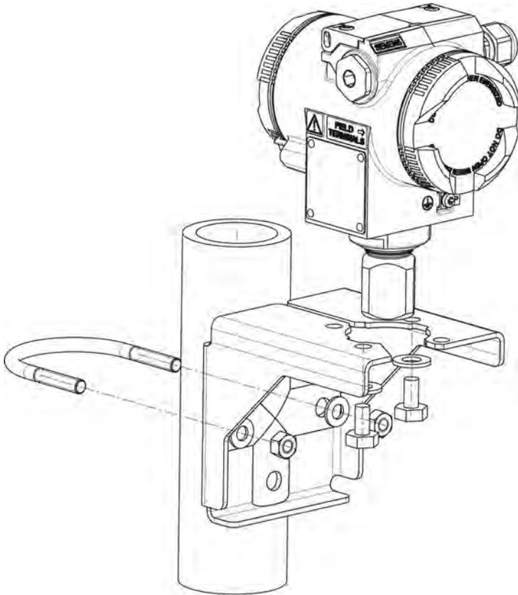
Figure 3-1 Fastening the transmitter on the mounting bracket
